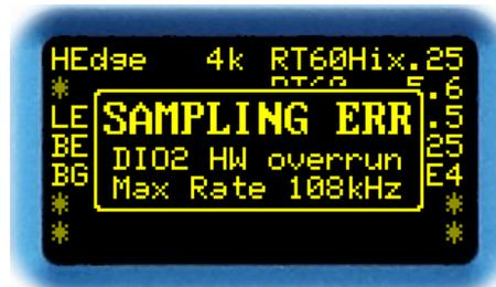
Fig. 18: Hardware sample rate error
