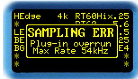
Fig. 17: Plug-in sample rate error
